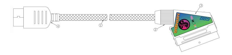
Mamba is a specially made Scart cable with individually shielded, impedance matching, 75 Ohm coaxial cables, so it delivers unparalleled audio and video quality. It's compatible with all Dreamcast revisions from every region, and supports all video resolutions from 480i to 480p. So, you can play every game released in RGB or VGA modes. With the MAMBA, you'll experience your favorite Dreamcast games like never before, with crystal clear graphics and immersive sound.
