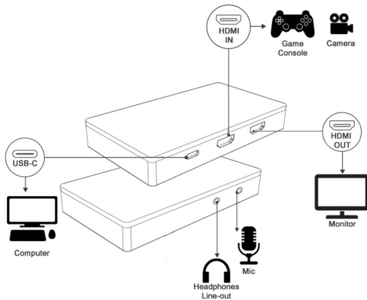
1. USB3.0 Type-C port: Connect the Prodigy to your computer by using the provided USB 3.0 cable, its indicator led will illuminate yellow when the capture software is running.
