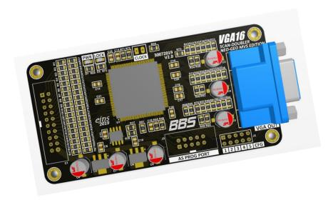
VGA16 samples NEO-GEO's 3x5 Bit Digital RGB, DAK and SHD signals before going to the resistor divider DACs. This data is level shifted and fed to the FPGA for further processing. FPGA captures every scanline and sends to VGA output interface twice. Since NEO-GEO's original video output is NTSC (~30FPS, interlaced, 262.5 lines per field), by using this technic, we are able to generate a 640x480 @60Hz Progressive VGA signal.
